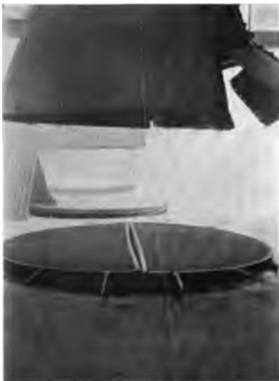
Fig. 3. Guard for Cupola during re-lining.*
